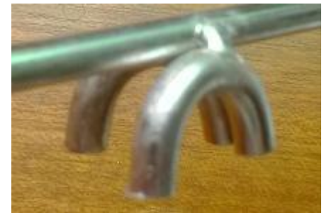
The claw fasten the top of the bottle & press it to let gel out
