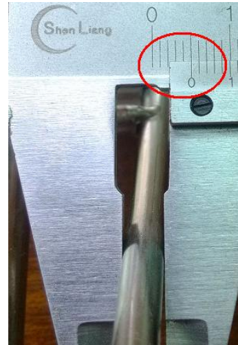
Strong lever with diameter 5mm, made by 304 stainless steel.
