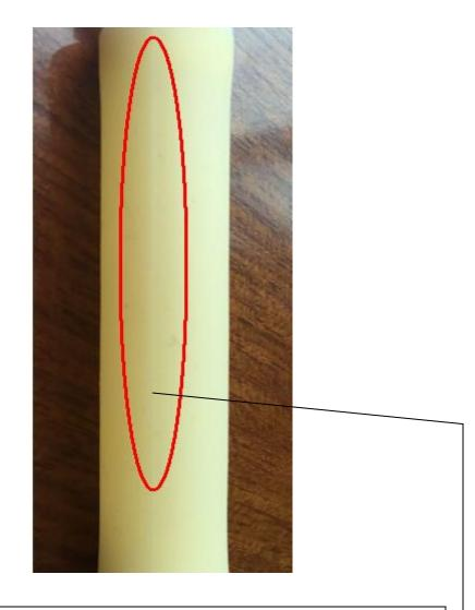
Other nozzle supplier, the technology of nozzle has trace line that has the venture on broken in the usage.
